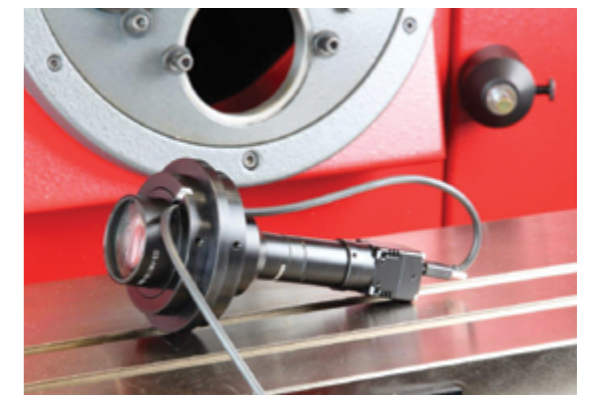
TOV2 Video camera for Optical Comparators work with M3 software
